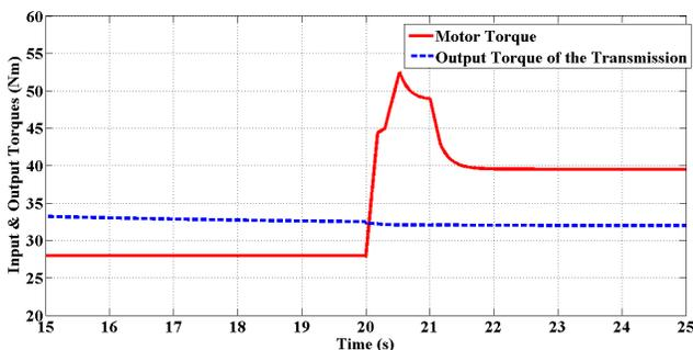
Fig. 4. Motor Torque and Output Torque
