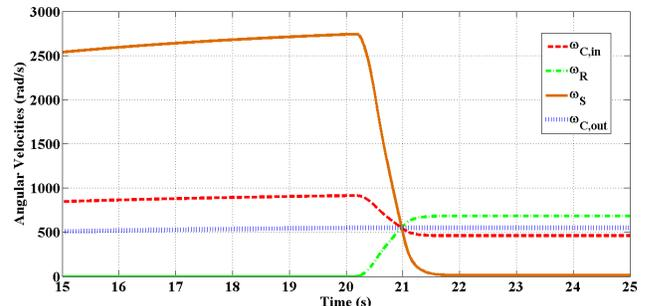
Fig. 2. Angular Velocities of the Input, Output, Ring and Sun
