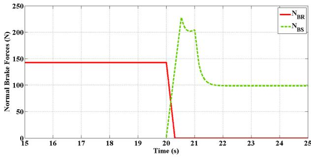
Fig. 3. Normal Braking Forces of the Ring and Sun
